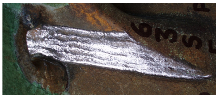
Fig 20 Multi-pass weld after multi-striker treatment
