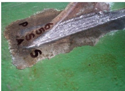
Fig 19 UP treated weld flange
