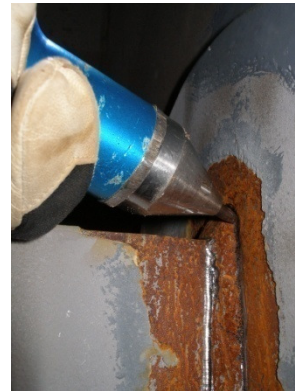
Fig 13 Weld toe UP Ø 3 mm
