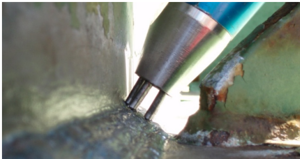
Fig 17 Multi-striker working head
